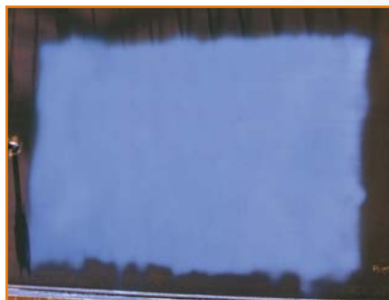
15 minutes blasting with GMA Garnet: 60ft 2 blasted – 75kg used. Amazing!
