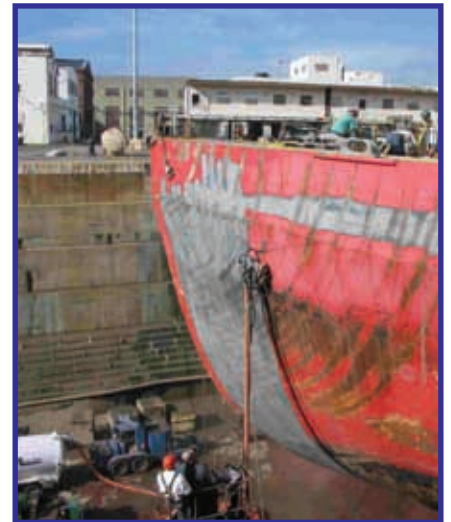
The SRT-10 Crawler maintains a tight seal against the ship's hull by high vacuum.
