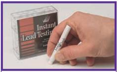
Lead Check Swabs This is how you check for the presence of lead in paint on structures. A simple, quick, qualitative test. Also available to test for chromates.
