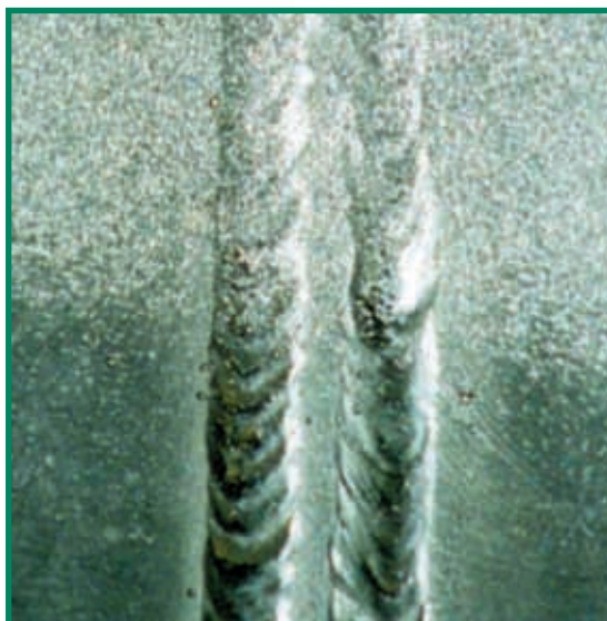
Profile after blasting gives excellent surface for painting.
