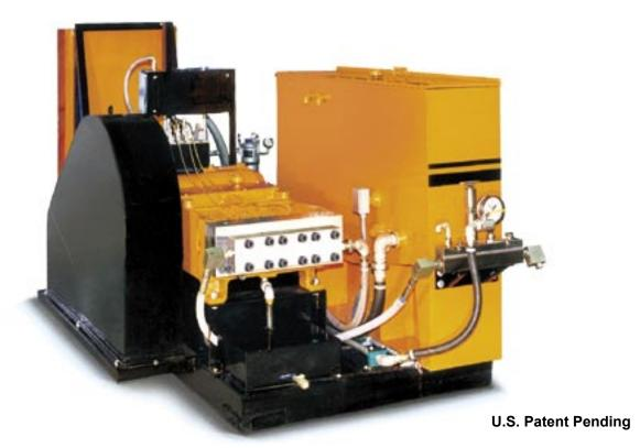
NLB's newest line of waterjetting units are built around the innovative model 225 convertible pump. This pump, with its quick-change, in-line fluid end design, has fewer parts for increased operating efficiency and simpler maintenance. And, it requires only a simple conversion kit to operate at pressures between 8,000 psi (552 bar) and 24,000 psi (1,680 bar).
