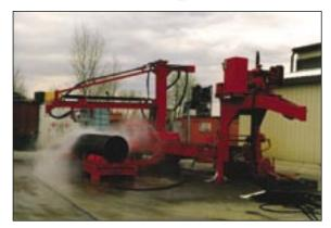
The pressure and flow produced by the NLB 350 Series pumps makes it ideal for use with NLB's shellside cleaners.
