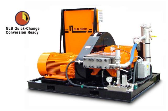
NLB's newest line of water jetting units are built around the innovative Model 605 Series convertible pump. This pump, with its quick-change, in-line fluid end design, has fewer parts for increased operating efficiency and easier maintenance. And, it requires only a simple conversion kit to operate at pressures between 4,000 psi (275 bar) and 20,000 psi (1,400 bar).
