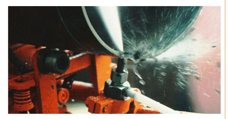
NLB high-pressure water-jet abrasive cutting systems cut metal, concrete, composites and many other hard materials. Operating at pressures of up to 40,000 psi, they can quickly and efficiently cut concrete and rebar, or inspection and service openings in petrochemical tanks.
