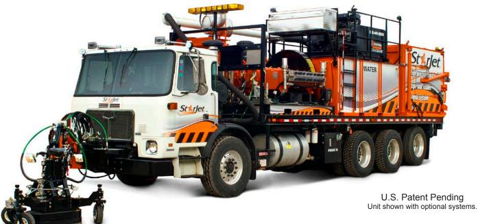
If you want to remove road or runway markings faster and more thoroughly than abrasive methods - without damaging the surface - you need an NLB water jetting system. NLB's StarJet™, allows operators to quickly and thoroughly remove stripes and other markings using nothing but the power of ultra-high pressure water.
