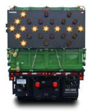
The 25 light traffic arrow board, along will all the other work lights, are completely controllable from within the cab.
