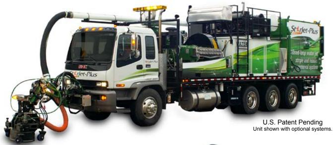
NLB's StarJet-Plus<sup>™</sup>, allows operators to remove more pavement marking or runway rubber per shift than ever before. It is the first ultra-high pressure water jet system with a closed loop, on-board vacuum and filtration system, so users can fill the water tank once and work all day without stopping to refill. This typically saves about two hours of downtime per 8-hour shift, speeding up project completion.
