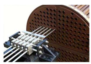
NLB's simple to operate lance pitch adjustment controls move each lance at the same time, ensuring that they are spaced correctly.
