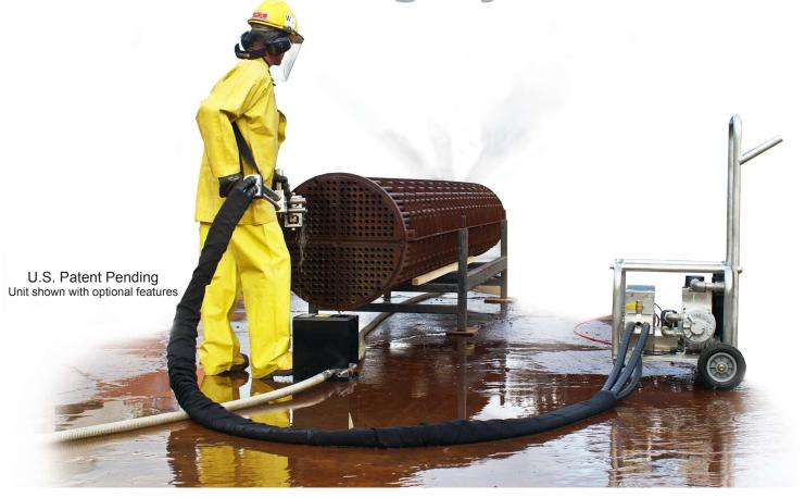
NLB's new Saflex line of semi-automated tube lancers are safe and effective tools for water jet cleaning the I.D. of tubes. They feature an all new hose drive system that is powerful enough to drive hoses with an O.D. range of 4 to 15 mm. at pressures to 40,000 psi.
