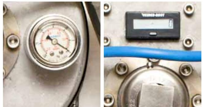
Easy to read displays like the vacuum gauge and RPM indicator are located directly on the SRT-6LT.
