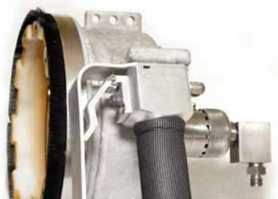
Each dual trigger configuration (one on each handle) ensures the operator always has both hands on the device during operation.
