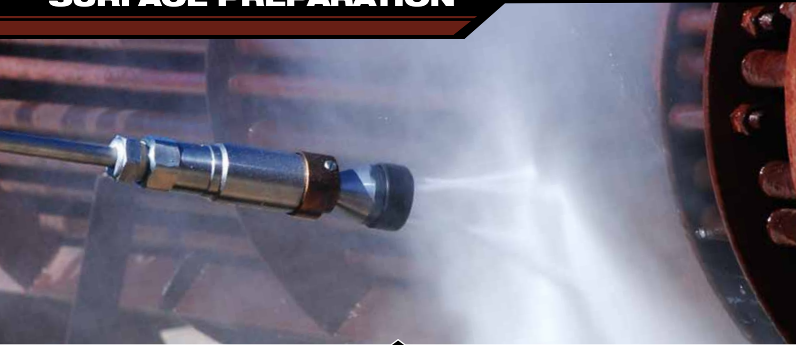
Self rotating, speed controlled, lightweight shotgun tools.
