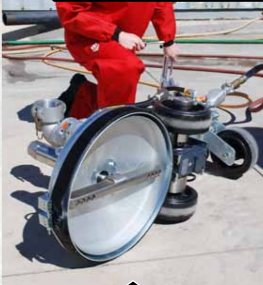
DECK BLASTER with eight-jet bar head.
