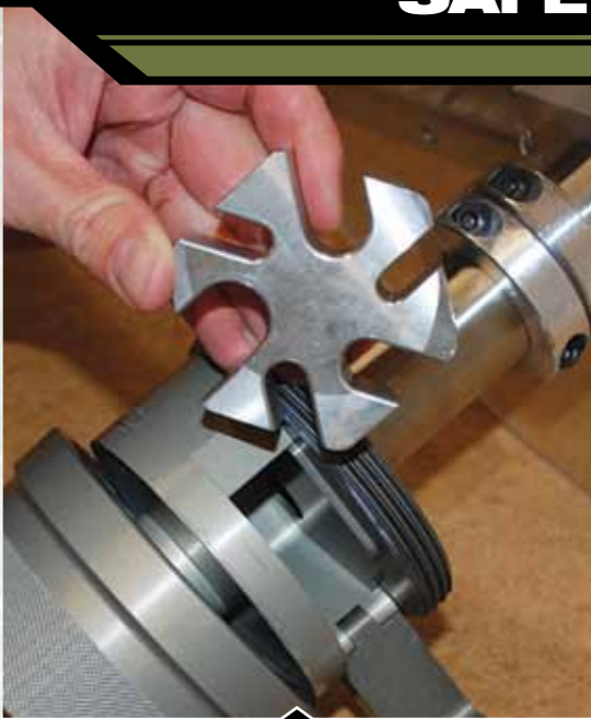
Collet adjusts easily for different hose sizes.
