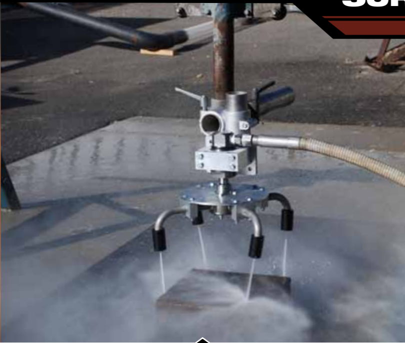
Radiused arms produce powerful and effective jets.
