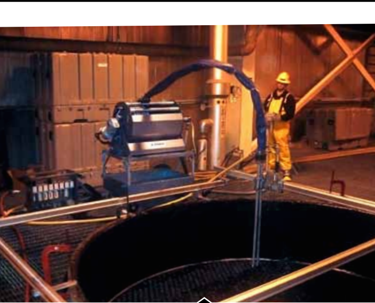
Remote Sabertooth controls keeps operator at a safe distance.
