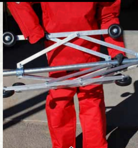
Centralizers prevent tool turn around.
