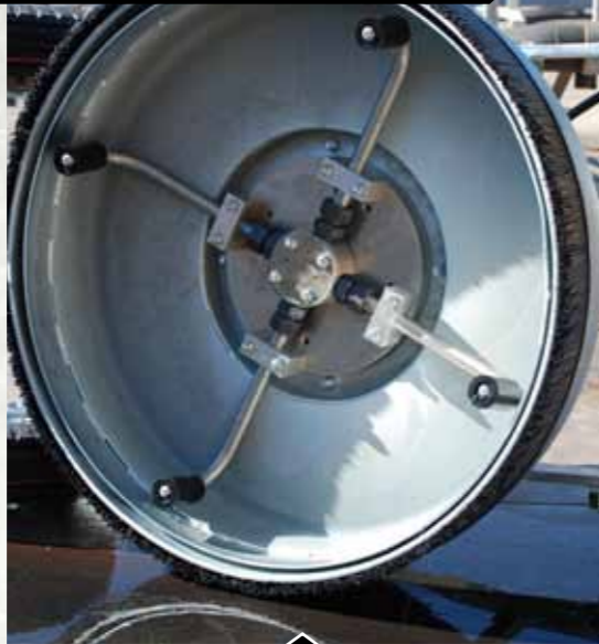
Radiused arms for free-spinning jets.
