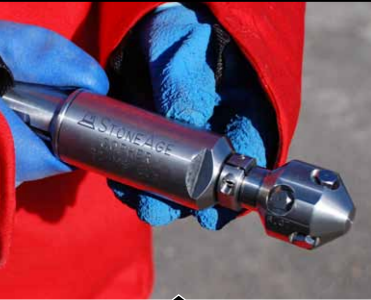
Powerful rotary tools for cleaning straight pipes 2" or larger.
