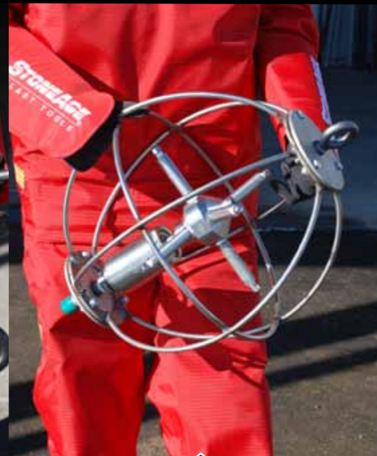
Cage styles are ideal for pipes with bends.
