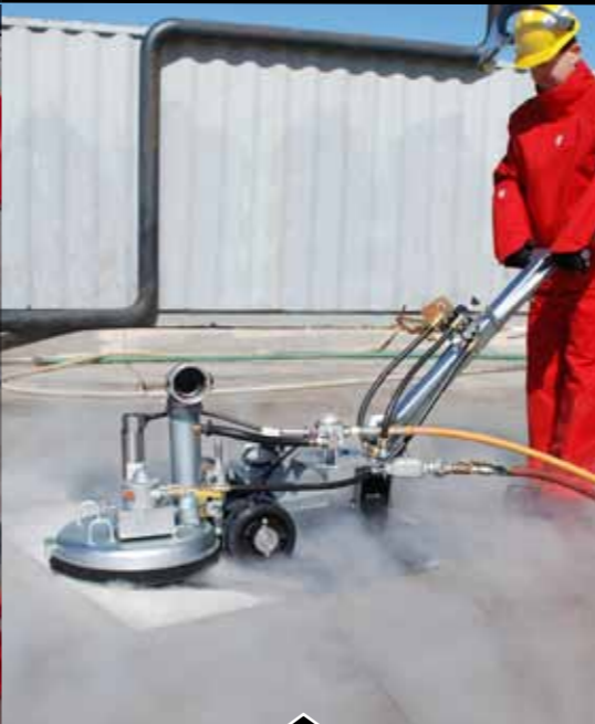
Adjustable rotation and traverse speed.
