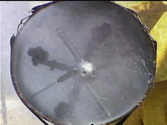
BJV cleaning pipe with four extension nipples.
